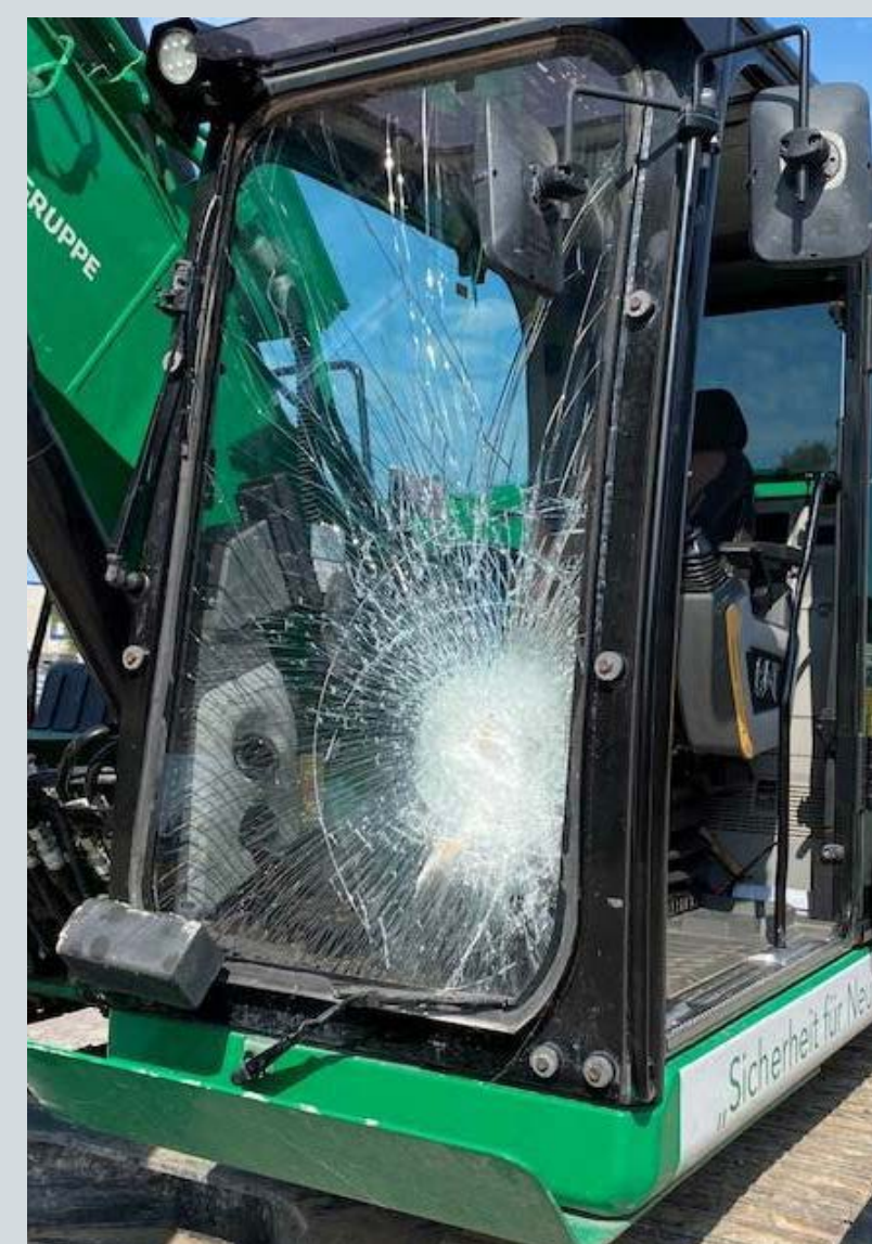
ARMORED PANE BEFORE ... ... AND AFTER BALLISTIC FIRING TEST
